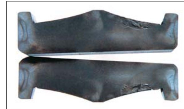
Part: Cross section of a fractured inner ring in a spherical roller bearing Symptom: Origin is directly beneath the raceway surface
