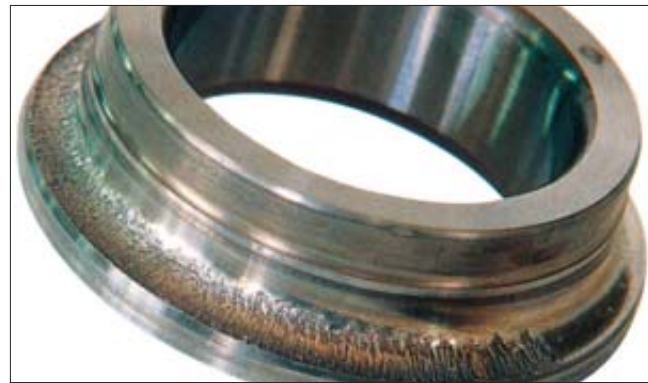
Part: Inner ring of an angular contact ball bearing Symptom: Flaking occurs around half of the circumference of the raceway surface Cause: Incorrect lubrication due to entry of cutting coolant into bearing
