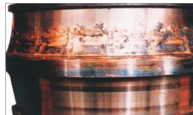
Part: Inner ring of a spherical roller bearing Symptom: Discoloration and melting of raceway; worn particles from the cage were rolled and attached to the raceway Cause: Insufficient lubrication
