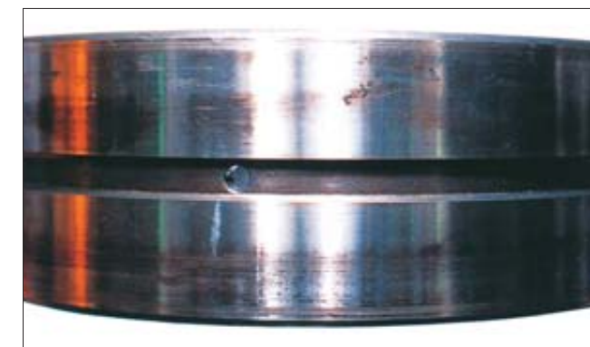
Part: Outer ring of a spherical roller bearing Symptom: Creep occurs over entire circumference of outside surface Cause: Loose fit between outer ring and housing
